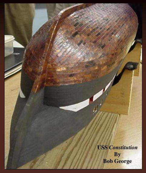
**Coloration was** achieved by placing the plates on a cookie sheet, which was covered with Reynolds Wrap. They were then "cooked" on a gas grill for 30 to 40 minutes.
