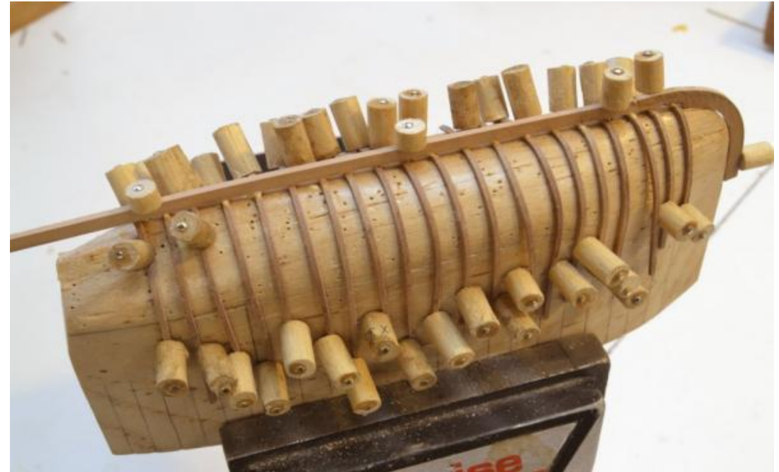
Contoured form to inside of ribs; Ed Tosti
